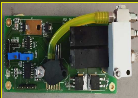
Vacuum and pressure regulator system
