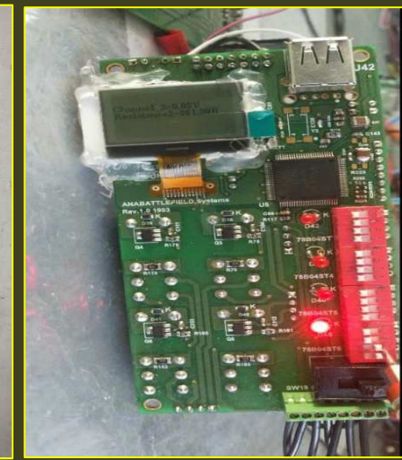
Earth Leakage detection & adding insulation system
