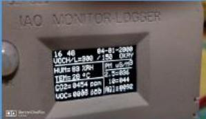
**Remote Air Quality Sensor (2-wire MODBUS 1km max)**
